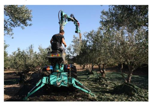
This machine is particularly helpful for the early harvest, because it avoids the damage that normal shaker machine can do when the tree is still in the full vegetative period.
